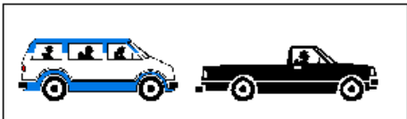
(LSIORB Class – Auto) FHWA Class 3 — 2 Axles, 4-Tire Single Units, Pickup or Van (With 1- or 2-Axle Trailers)
